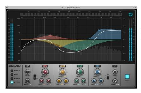
This is the Big and Bright curve for the J-200, which is already pretty big and bright. Again, the **G-Type** EQ works well; it adds more emphasis to the lows and highs while de-emphasizing the midrange. The "bigness" comes from a boost in the 100 – 200 Hz range. Lo Mid provides a general midrange cut to reduce any tendency toward "muddiness," while Hi Mid reduces the range
