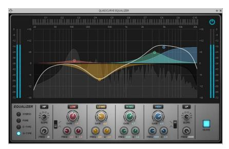
The Articulated preset (for the J-45) is useful when accompanying other instruments that occupy the midrange, particularly vocals. It brings out finger picking and gives more note definition by emphasizing the upper mids and highs, while reducing the midrange to leave more "space" for other instruments. The **G-Type** EQ seems to sound best for this applications.
