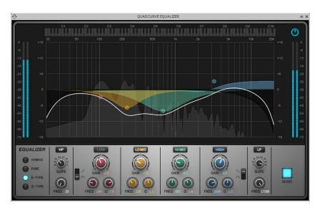
This shows the Rhythm Natural preset for the J-200. The main object is to lower two resonances from the piezo pickup, while retaining the low end and giving a slight boost in the 5 – 10 kHz range, but rolling off gently above 10 kHz to reduce some of the unnaturally high frequencies contributed by typical piezo pickups. The preset results in a natural guitar sound, like what you
